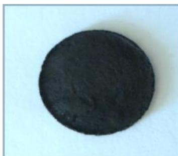
Figure 3. An example of an electrode made for a zinc-air battery model
